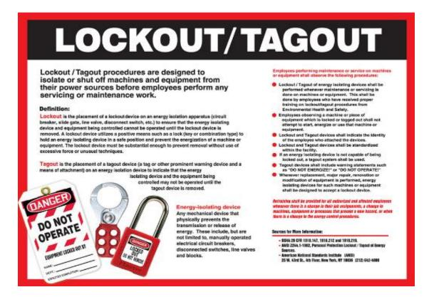
**Lockout-tagout** (LOTO) or lock and tag is a safety procedure which is used in industry and research settings to ensure that dangerous machines are properly shut off and not able to be started up again prior to the completion of maintenance or servicing work.
